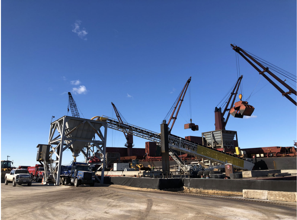
Figure 5. Ship unloading with conveyors and hoppers at Atlantic Salt in Staten Island, NY.
