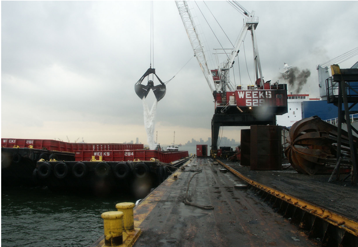
Figure 7. Crane barge unloading salt from vessel anchored in New York Harbor to bring to Atlantic Salt terminal in Staten Island, NY.
